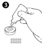
3 Place the InstantGold cap on the test cartridge. Dispense 12 drops of Universal Buffer onto the InstantGold cap and allow the solution to absorb completely.
