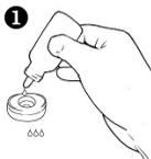
1 Apply 3 drops of Universal Buffer to the center of the test cartridge. Allow the buffer to absorb completely.
